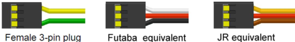
Only two of the four signal wires are needed to control the Talon SRX with PWM. Do not connect two PWM connectors to a single Talon SRX. The two signal wires not used should be electrically isolated using tape or heat shrink tubing and bundled out of the way.
